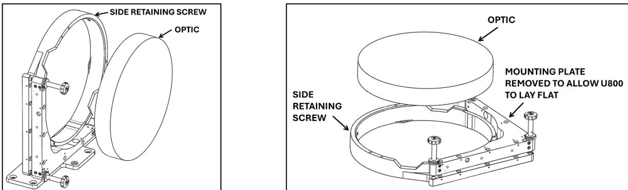
**STEP 3:** Re-install the brackets and finger-tighten the Optic Retaining Set Screws with included 3 mm Thumb Hex Tool.
