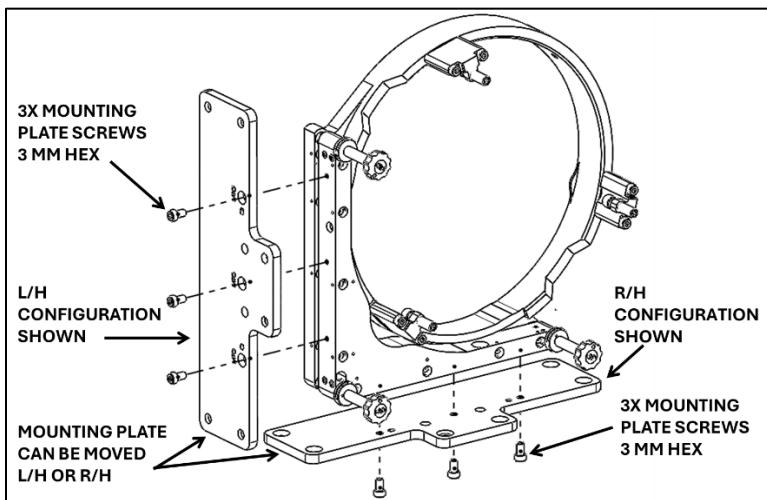
To switch between left-hand and right-hand configurations, the mounting plate must be repositioned. The figure shows the location of the three screws that need to be removed to make this change (3 mm Allen included with U800-AC model). The plate also needs to be removed when swapping out AJS adjusters.
