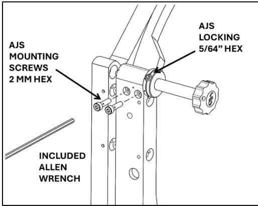
The included 2 mm (5/64") Allen wrench secures the AJS mounting screws and can also be used to engage the AJS flexure lock.
