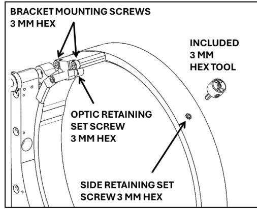
The included 3 mm hex tool fits the optic retaining soft-tip set screws, the side optic retaining screw, and the bracket mounting screws.
